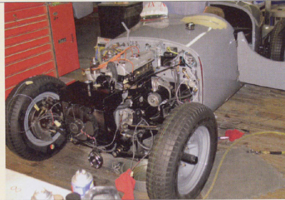
During the teardown it was discovered that during the original restoration, all the wiring was made the same color. Suffice it to say that's not the way it is now.
