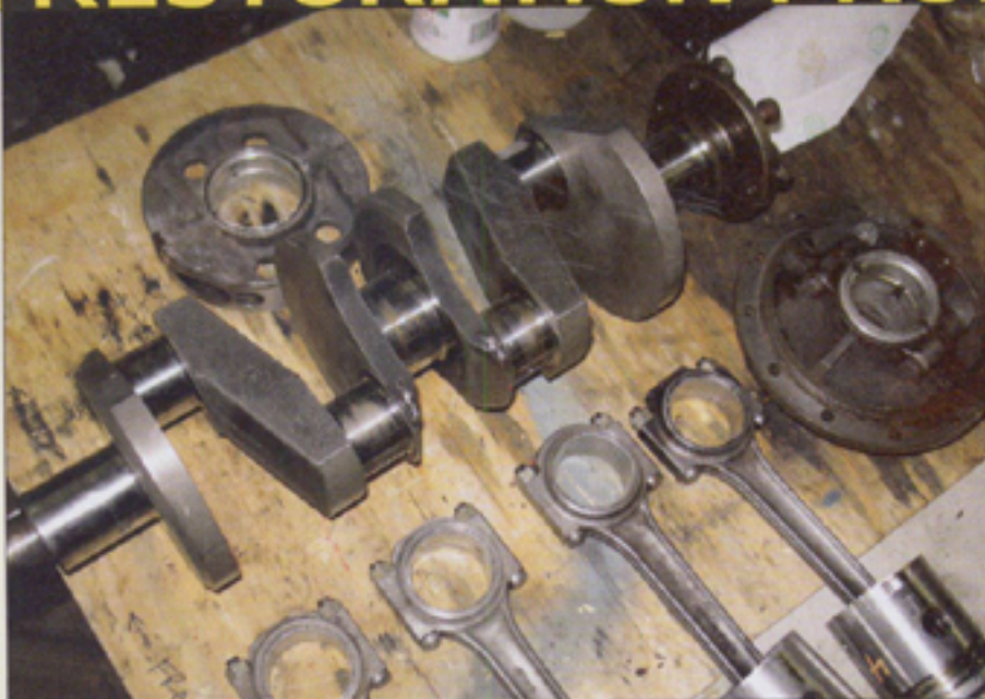
At some point in its history, the main journal bearing surfaces had been machined past tolerances, requiring babbitt bearings to be poured in the original bearings' place.
