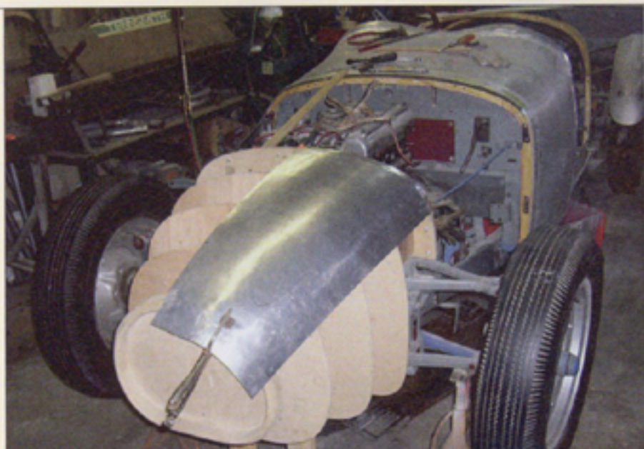
After scanning original period photographs of the car, the restoration team overlaid a grid that helped to construct a plywood buck to create the Connaught's nose.
