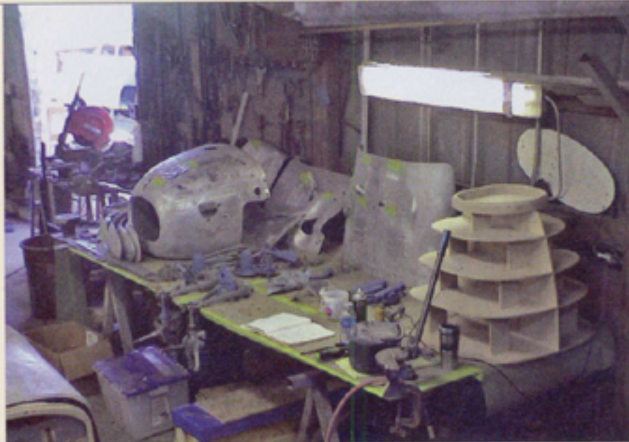
The finished nose is at the back of the bench, following weeks of metalwork. Note also the newly constructed cycle fenders, hood panel and engine side panels.
