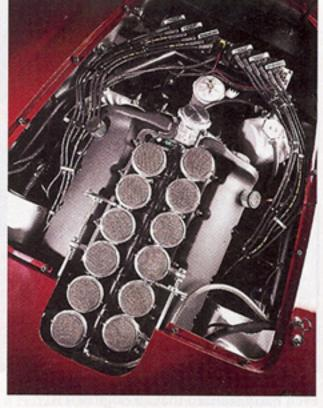
and 480 lb-ft of torque by the factory and Korman Autoworks. To mimic the Webers, a custom Hilborn-style fuel-injection system features a dozen stacks.
